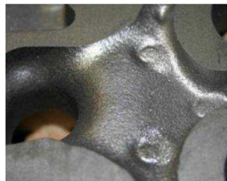
Fig. 7 : Casting surface with MIRATEC TS
