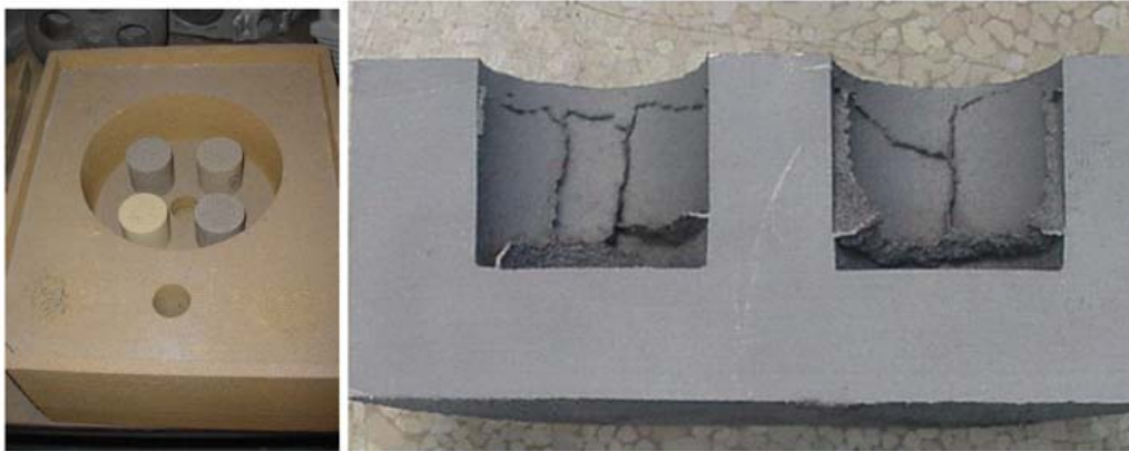
Fig. 3 : The 2 x 2 inch cores and mould (left) and a sectioned casting (right) exhibiting the veining defect
