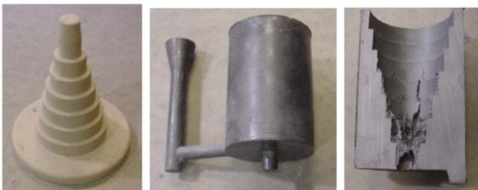
Fig. 2 : The Step Cone core (left), casting (center), and sectioned casting (right)
