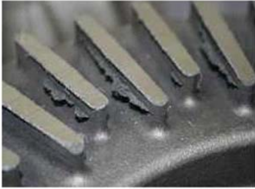
Fig. 4 : Brake disk with veining
