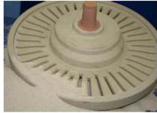
Fig. 5 : MIRATEC BD prevent in the parting line veining defect
