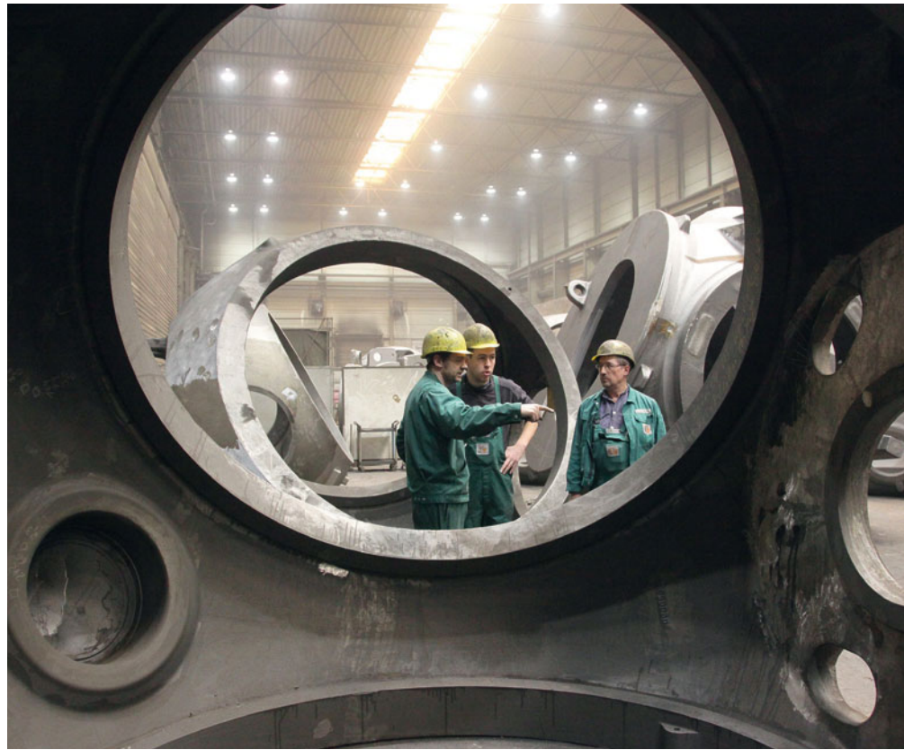
Figure 1: Among other products rotor blades, frames and generator housings for wind power systems are cast at the Torgelow foundry
