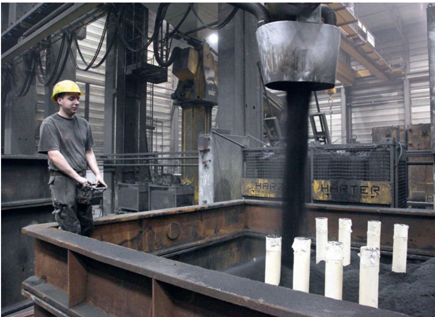
Figure 3: The right mixture of furan resin for large-scale cast parts is an indispensable success factor
